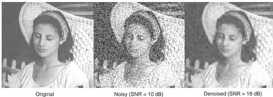
Figure 6. Wavelet shrinkage denoising with 'SUR,' DROLA (10; 5), n = 464 \times 320 , L = 4 .
