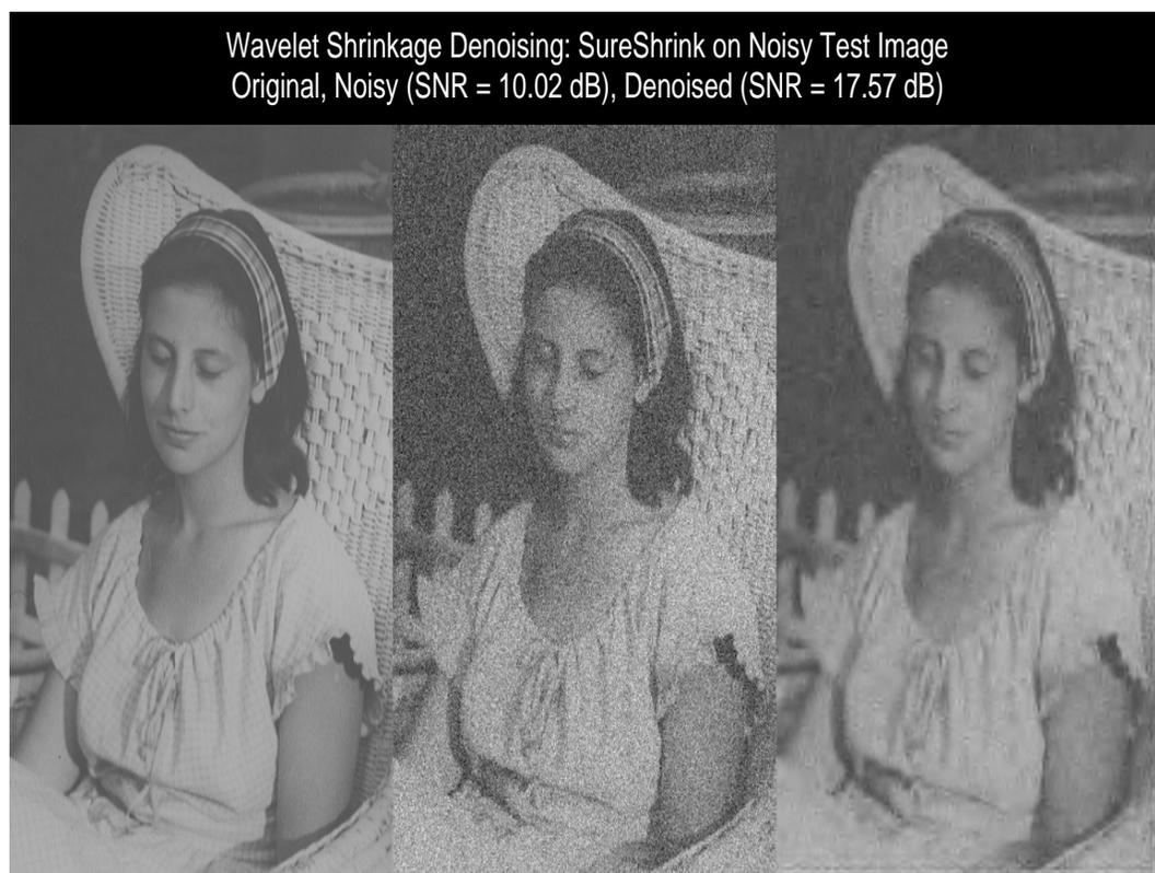
Figure 6: Wavelet shrinkage denoising: 'Elaine', 'SUR',  $\mathbf{n} = [464, 320]$ ,  $L = 4$ , DROLA(10;5).
